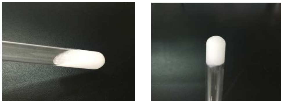
Figure 1. Gel under different temperature conditions (left for the gel state at room temperature, the right is the gel state after transformation under the conditions of 37 °C)
